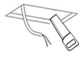
2.Adjust the height of the embedded parts to be flush with the gypsum board. place the embedded parts
