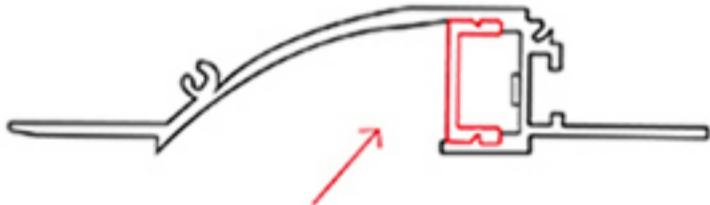
5. Connect the power, use the screws to fix the aluminum profile
