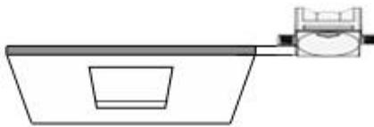
2. Adjust the embedded part height, flush with the gypsum ceiling/drywall
