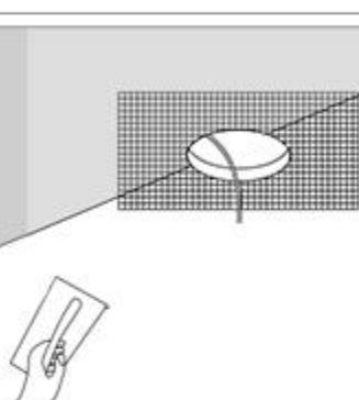
2. Plaste-mesh-putty-paint, finish the ceiling
