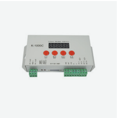
Model: K-1000C Single port SD card offline controller Support DMX/SPI Power supply voltage: DC5-24V Support multiple cascades Number of controllable ICs: 1024 / DMX512: 300 Support IC: most SPI/DMX512 Support DIY programming, with supporting software
