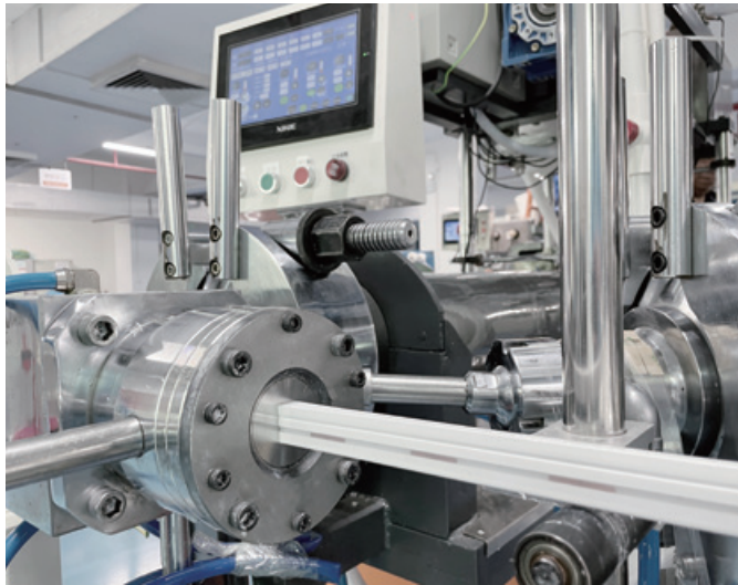
6 Production lines of silicone co-extrusion
