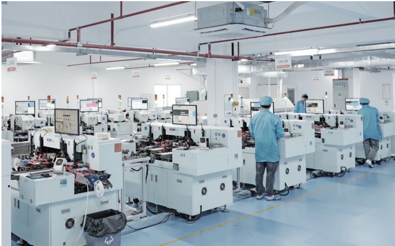
10 Sets high speed SMT machines and 15 sets COB Die bonder machines
