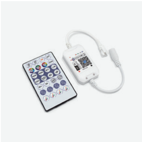
Model: BWCAS-HCP1-R28A4 Voice control controller type A Only support SPI light strip/RGB/RGBW Power supply voltage: DC5-24V Number of controllable ICs: 2048 Support IC: WS2812B, WS2815B, SM16703, SM16703RGBW, WS16704, WS2811, UCS1903, SK6812, SK6812RGBW, INK1003, UCS2904B, UCS2904RGBW
